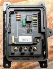
Power Control Module
